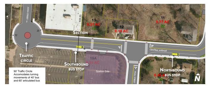
Recommendations for this area include relocating both the northbound and southbound 9-Town Transit stops to the south side of Central Avenue. Sidewalks at the bus stops would be expanded to eight feet, and a nine foot wide bus stop/shoulder would be provided to remove buses from traffic lanes when stopped. Northbound buses would stop on Central Avenue immediately east of Hull Street while southbound buses would stop on Central Avenue west of Hull Street and at the planned station site.
