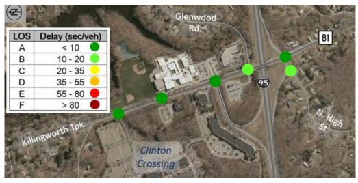
Figure 3.8: AM Peak Level of Service (LOS) at Signalized Intersections
