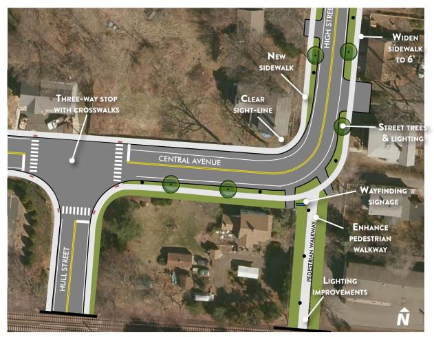
Recommendations for this segment of the corridor include the addition of a three-way stop at the intersection of Central Avenue and Hull Street. This would improve pedestrian crossing safety and reduce turning movement conflicts. The three-way stop would be accompanied by crosswalks at all approaches.
