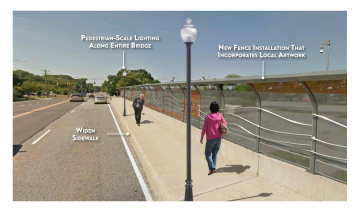
Improvements in this area include widening the sidewalk and adding pedestrian area lighting. Lighting would be the same throughout Route 81 and would be a unifying element in the corridor. The existing chain link fence should be replaced with a decorative barrier or a new colored vinyl coated chain link fence. These improvements would encourage walking trips between the Clinton Crossing area and Downtown Clinton.
