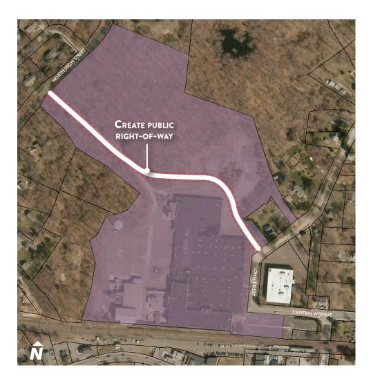
Provide a public right-of-way and roadway through the Unilever property connecting John Street and North High Street. The new roadway would provide an alternative to Route 1 for local trips and could potentially reduce public safety response times in the immediate area. The roadway would also have the benefit of making the Unilever site more accessible to the general public.
