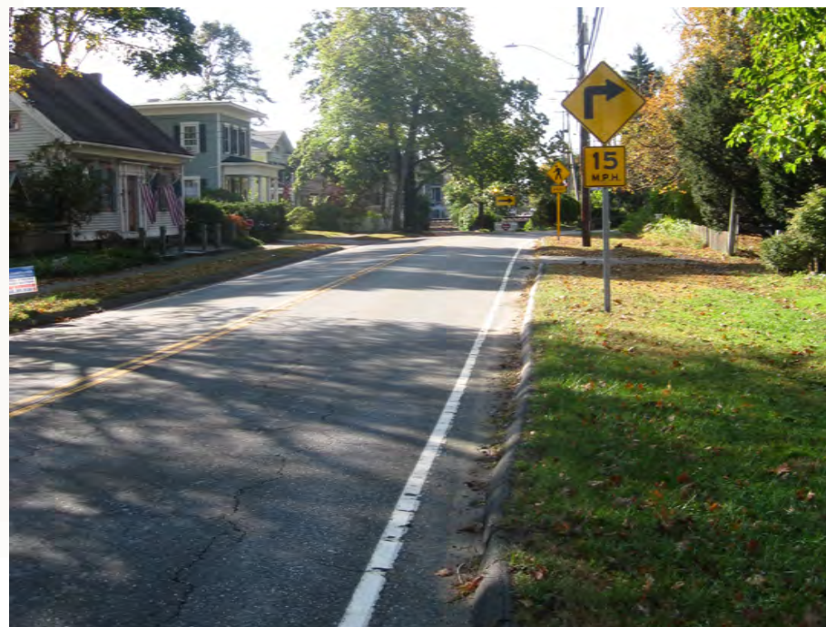
Advance turn right warning sign with speed placard and advance pedestrian crossing signage. Source: VN Engineers
