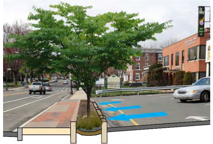
Pitch pavement toward bioswales & planted areas
